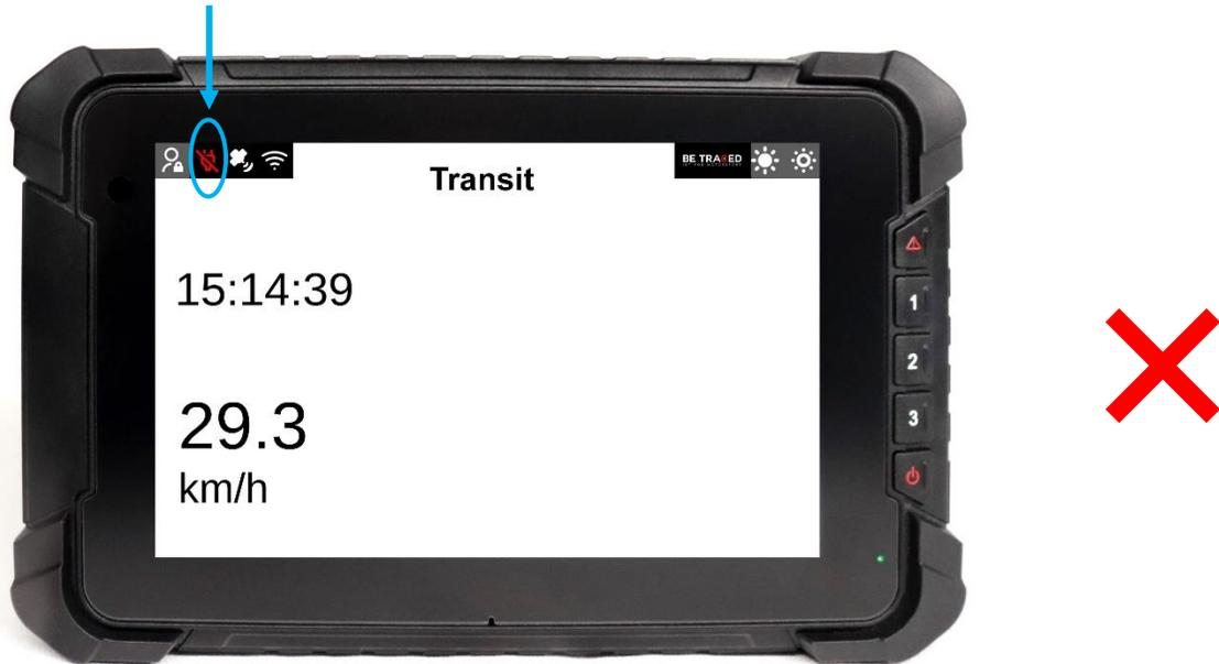
Figure 2 - Red power indicator light: device not powered
