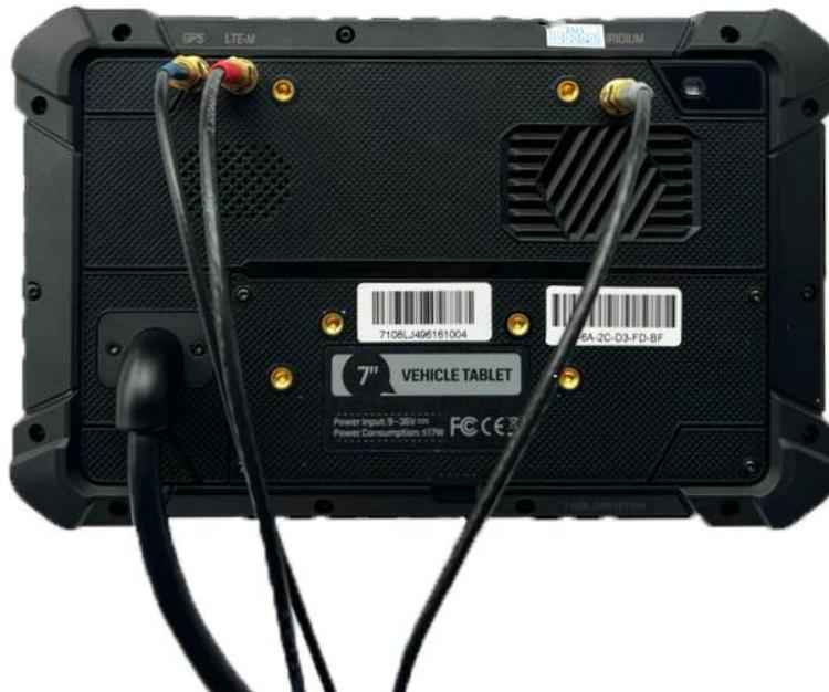
Figure 3 - Antenna connectors
