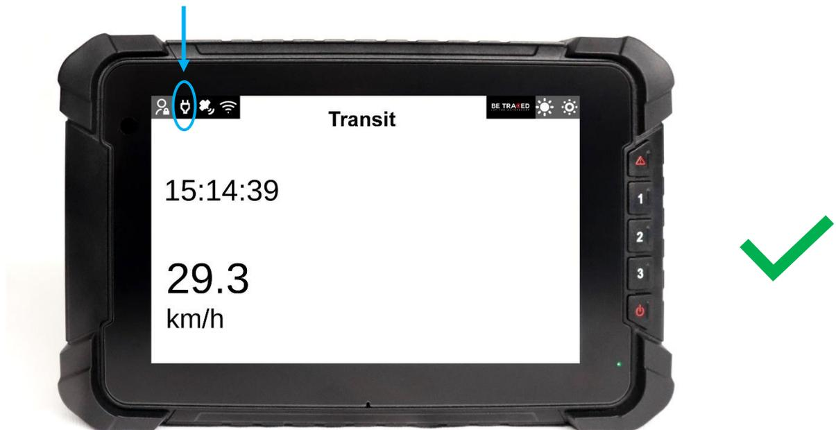
Figure 1 - White power light: device powered correctly
